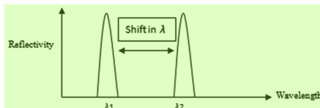
Fig. 7 Wavelength shift due to external perturbation. 7
